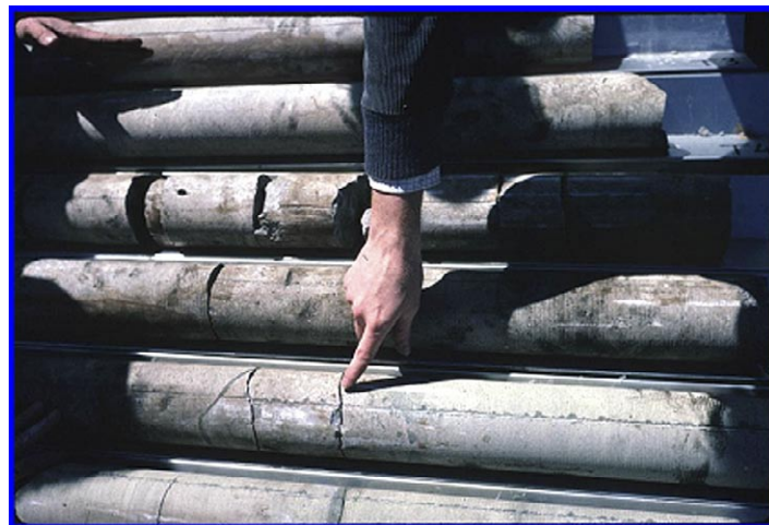
Part of 4” drill core retrieved from ~8000 ft depth
